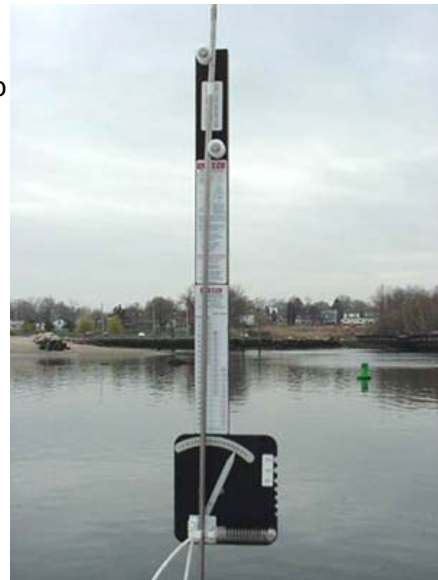
Measuring Rig Tension with the RT-11m Gauge
